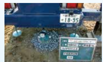
Post testing (plate loading test) is always performed.
